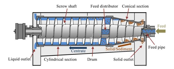
Decanter centrifuge is mainly composed of cylinder-cone drum, screw shaft, differential system, bearing seats, frame, cover, main and auxiliary motors and electrical control system. The main motor
